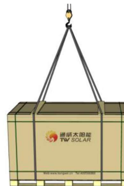
Figure 6 Schematic diagram of Module lifting
