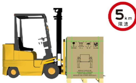
Figure 8 Note the speed of the forklift
