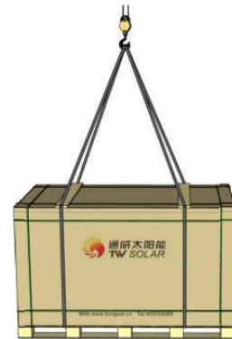
Figure 5 Schematic diagram of Module lifting
